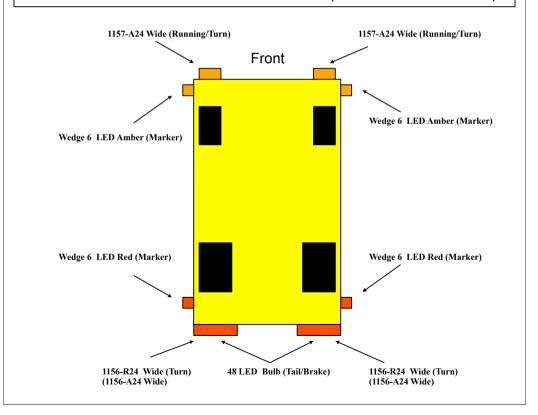
1) Remove the four screws securing the tail light lenses to the main housing. After the lenses have been removed you will see three separate bulbs in each housing. The upper bulb is a dual filament brake and tail light bulb. The lower bulb nearest the outside of the car is a single filament turn indicator bulb. The lower bulb nearest the center of the car is the back-up light. Retain your original back-up bulbs as the kit does not replace the back-up lights.
