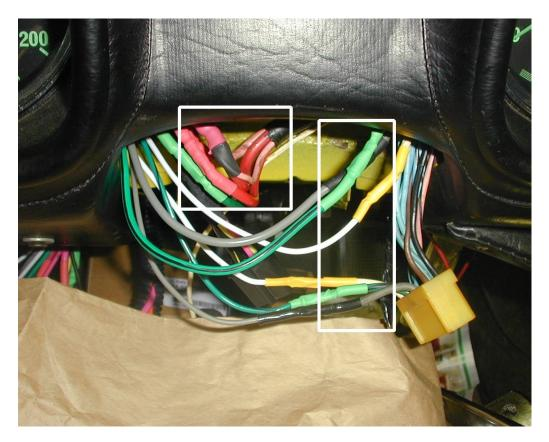
21) The left rectangle shows the power output of the ignition switch relays connected to the harness-end of our harness wires. The right rectangle shows the Hi/Low beam power wires connected to the harness-end of the cut wires *and* the control wires connected to the big yellow connector which leads to the steering column switch. Notice I got fancy by using colored heat shrink tubing obtained from Fry's Electronics.
