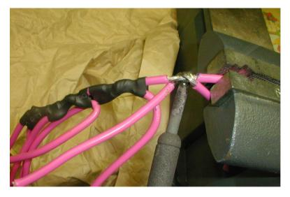
12) The pink 10-gauge power buss supplying current to all (except the light interrupt relay) is shown being soldered to a jumper pair.
