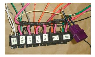
14) Close-up of the finished relay module with Bosch type bases and 10-gauge pink power buss installed along with the other wires and the fuse. Note the permanent labels for each relay base, the relays have not yet been installed.
