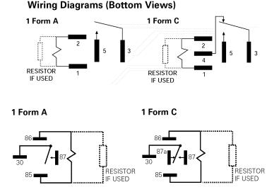
10) ISO (similar to SAE, but electrical) **micro**-relay, top, and **mini**-relay, bottom, terminals are an industry standard configuration.
