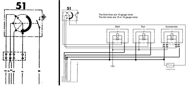
3) The ignition switch terminal strip is shown as the dashed box in the left diagram above.
