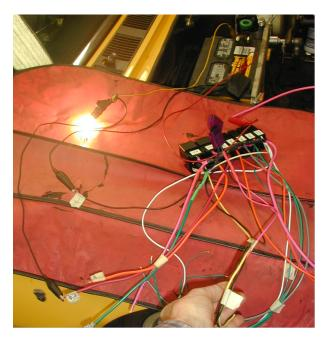
18) I took the module over to the car and did a bench test of all the circuits prior to installing it in the car. This tests all the relays and soldered terminations for correct operation. I used a test light made from a #1156 taillight bulb for my load.
