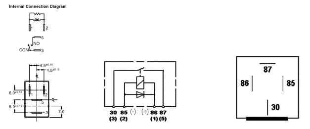
9) On the left is an ISO **micro**-relay with a resistor across the coil, and on the right is a **mini**-relay with diode across the coils. Both views are looking at the bottom of the relay. Both relays use the same 2 conventions to label the terminals, either 1 through 5 nomenclature or the 30, 85,86, and 87 nomenclature . Other types of relays are available, such as, ISO 280 micro and ISO 280 ultra micro. They do not seem to be as widely available at this time so I did not use them.
