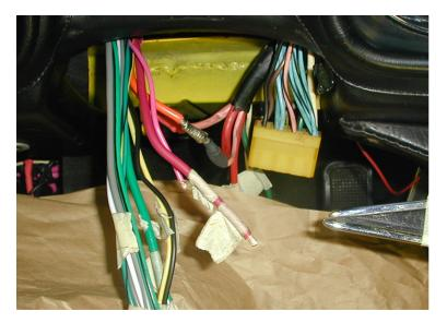
19) The Ignition and Hi/Low switch bundles coming down to the top of the steering column. The Harness-ends of the Ignition Switch wires are shown in the process of being soldered. The heat shrink has, not yet, been slid down over the soldered butt connector. The headlight wires above the yellow connector have not yet been cut. *Note* - masking tape is used to label the wires and butcher paper to protect the steering column.
