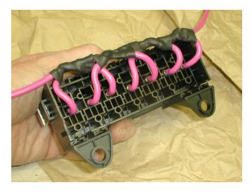
13) You can see it is difficult to bend the 10-gauge wire. I had to get creative and alternate the wires, connecting the 1st soldered jumper to relays #1 and #3. This photo is of the Hella relay block which was ultimately not used, but the 10-gauge buss was resoldered with new terminals and reused.
