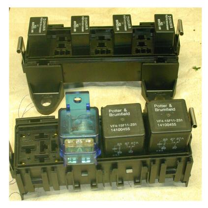
7) The Hella 7-position **micro** relay base (top) was not sturdy. The Hella 4-position **mini** relay base (bottom) seemed sturdier but not used. Note the blue Hella relay with integral fuse holder, which I felt was not desired in this application.
