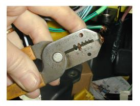
5) I used a precision wire stripper to be able to accurately measure wire gauge on the Pantera harness.
