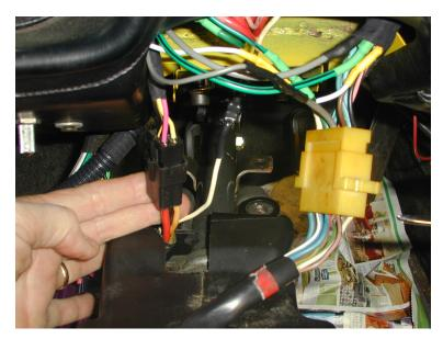
20) The 18-gauge control wires from the relay coils are routed to the new 4 pin Packard connector which connects them to the wires leading to the ignition switch. The Hi/Low beam relays are shown connected into the wiring just above the yellow connector. Note - the white wire has it's own connector.
