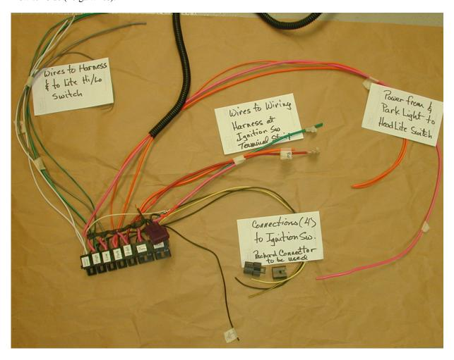
17) The wired relay module - I labeled the 3 bundles (the ignition switch wires are shown as 2 bundles)
