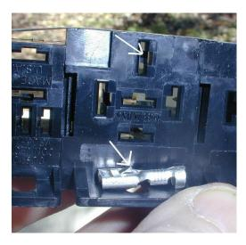
15) When the terminal is stabbed into the back side of the relay, it's barb, lower arrow, snaps into a recess, upper arrow, holding it firmly in place. Same with the Packard 4-pin connector female terminals. The connector's 4-pin male terminals are different. This is a better arrangement than the Hella micro bases.
