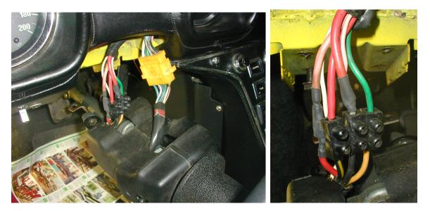
1) Left photo - The black ignition switch terminal strip is shown on the left side of the photo, and the yellow 8-pin connector for the lights and turn switch is on the right.
