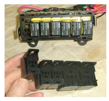
8) Panel mount Bosch type relay bases with tang and slot on the side of each base can connect 2 or more mini and micro bases together to make you own rugged multi-relay base containing both relay sizes. The Hella unit is at top of photo.
