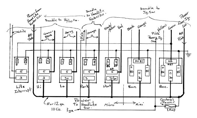
6) Above is a diagram of the wired relay module - as viewed from below, or the terminal side of the bases
